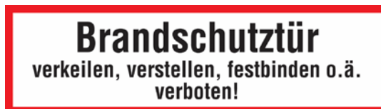
Picture 2 Marking of Fire and Smoke Protection Doors
